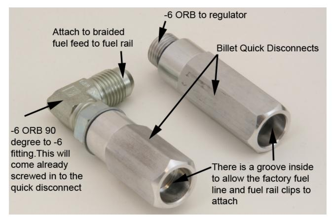
Attach the bracket, necessary fittings, and fuel pressure gauge to the regulator as shown in the following pictures. Connect the quick disconnect fitting to the factory feed line at the firewall. (you might want to use some WD-40 or silicone lubricant on the fitting to allow it to slide on a little easier). You might want to wait to attach the bracket to the car as you'll want to have the ability to move the parts around while you're connecting everything.
