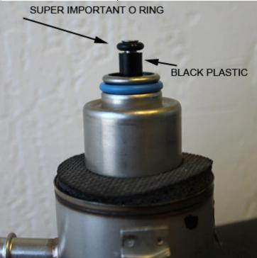
If while pressing in your block off bushing, your BLACK PLASTIC has been pushed down as well, and does not resemble the above picture, then use a second supplied SUPER IMPORTANT O RING. Double stacking these o rings is completely necessary to hold one in the proper location. IF YOUR BLACK PLASTIC HAS NOT MOVED WHEN PRESSING IN YOUR BLOCK OFF BUSHING, THERE IS NO NEED FOR ANY EXTRA O RINGS.
