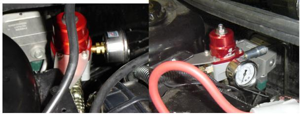
Before you start the car, turn the key to the "on" position five to ten times every 20 seconds to prime the system. Check all connections and make certain there are no fuel leaks at any of the fittings. Start the vehicle and let idle for about 10 minutes, keeping an eye out for any leaks at the fittings. Before you operate your vehicle follow this procedure each and every time you start your vehicle to ensure that every connection is tight.
