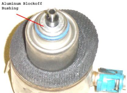
Please note that there is a super important o ring at the tip of the factory regulator. If your factory regulator does not have the o ring still attached to the tip, you need to inspect the canister and fish it out. If you do not have the o ring anymore, we have supplied a new SUPER IMPORTANT O RING. Note that before reinstalling the regulator; make sure it looks like the picture below.
